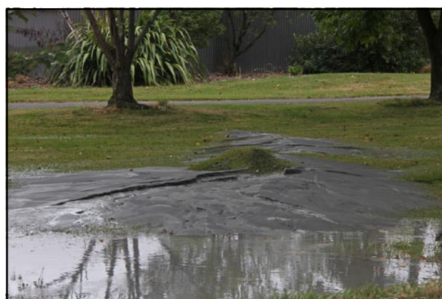
Figure 2. A silt volcano built on a grass verge by water and sediment extruded due to liquefaction of the ground when vibrated during the earthquake.
